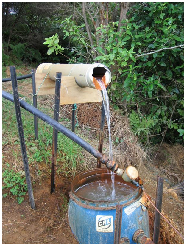
Fig. 7 Weirs and barrel 5 in the oxygenation cascade showing the siphon hose between the barrel and settling pond 1 with attached automatic flushing valve
